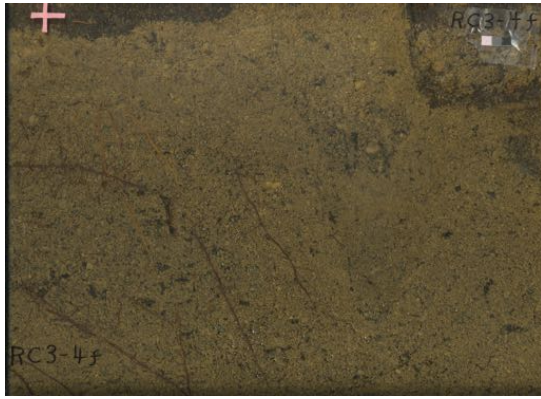
Fig. 1: An example of soil image taken by a flatbed scanner. Gray-scaled balance cards are embedded on the scanner and they are also imaged.
