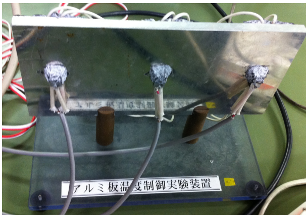
Fig. 2: Aluminum Plate Temperature Control Experimental Device
