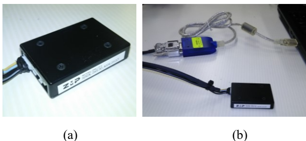
Fig. 1: ZMP IMU-Z nine-axis motion sensor, (a) sensor module, and (b) with CANUSB adapter.
