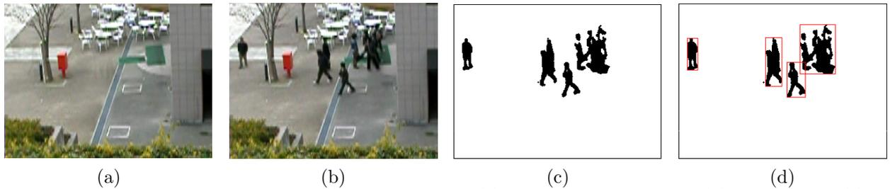
Fig. 2: Images used and processed in the proposed method. (a) The background image, (b) Input image, (c) The obtained image through the subtraction and binarization processes, and (d) The labeled groups of pedestrians with rectangles attached
