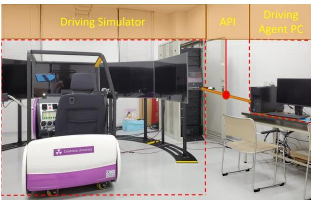
Fig. 2: Overview of experimental system
