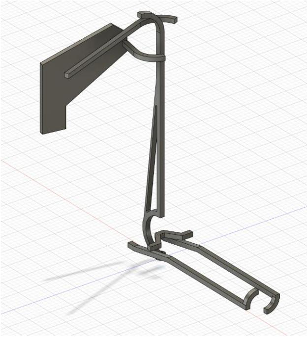
**Fig. 4** Newly created 3D model of the tensegrity arm.
