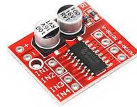
**Fig.7** mini-L298N Driver Board Module
