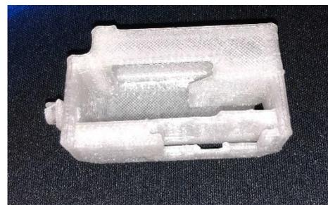
**Fig. 8** Actual 3D printed wire winder made of ABS material.
