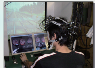
Measurement of Train Driver's Brain Activity by Near-Infrared Spectroscopy (NIRS)
