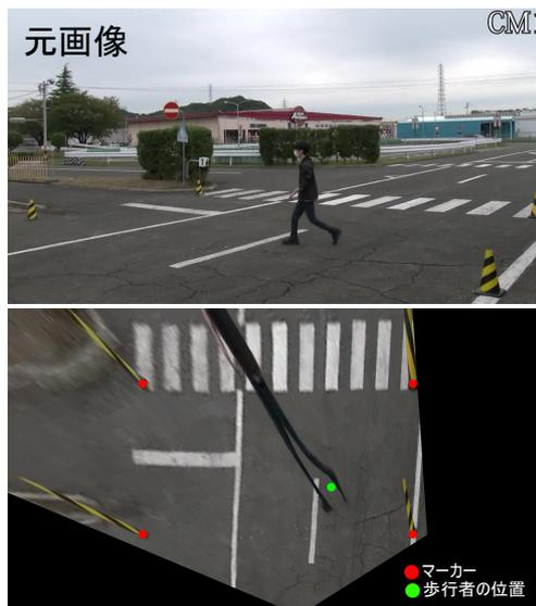
Fig. 6: An example of image projection using 4 key-points
